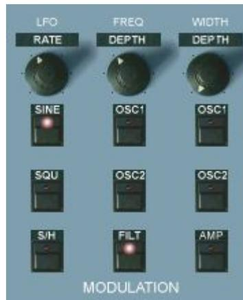
This is the section where the main LFO is controlled and routed to the desired modulation aims. For the modulation lever, there's a separate and independent sine LFO (rate control above levers). If wished, the modulation lever can be switched back to the main LFO as it is in the original device (ADDITIONAL FUNCTIONS SECTION, "Wheel LFO").
