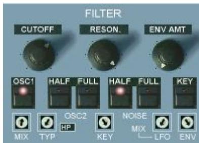
**HP (high pass):** Filters away the low frequency and leaves the high frequencies. Used for slim and thin sounding stuff to fit the arrangement/mix.
