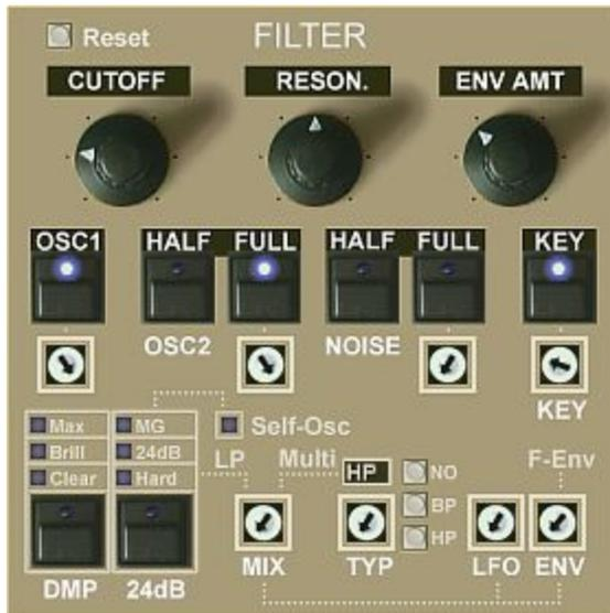
Dual filter design offering 10 filter types (7 lp + hp, bp, no)
